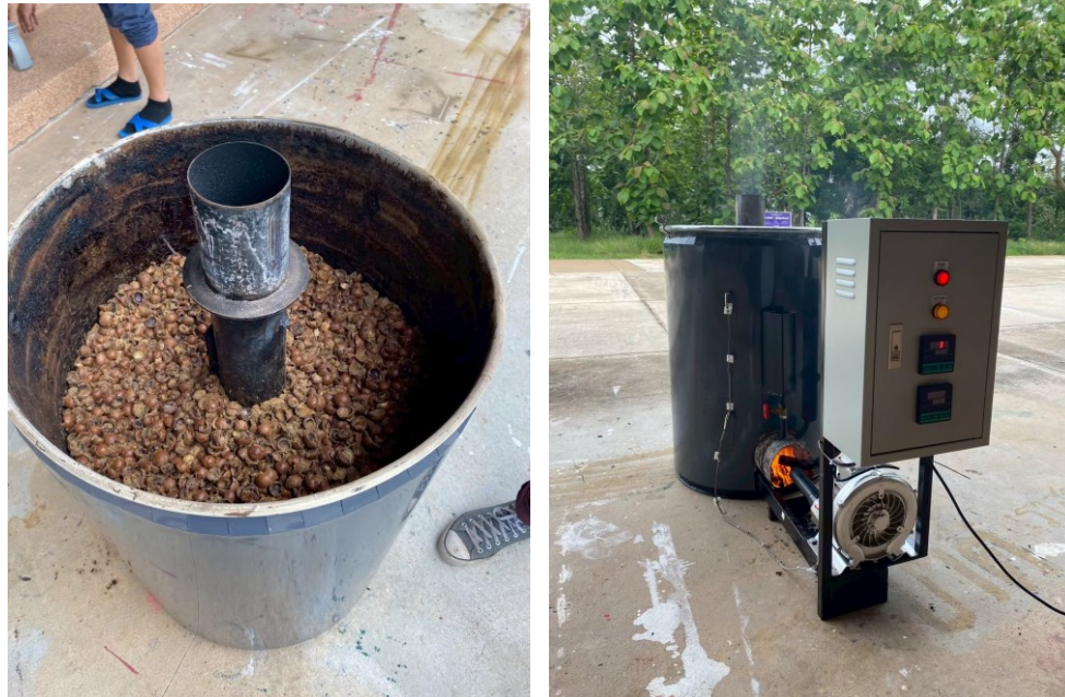
Figure 3 Preparation of macadamia nutshell feedstock (left) and experimental biochar production using the developed pyrolysis reactor (right).
