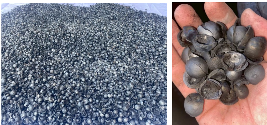
Figure 5. Biochar products obtained from the macadamia nutshell pyrolysis process, showing their characteristic porous structure and carbonized surface.
