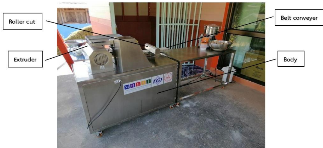
Figure 5 Prototype of semi-automatic banana stick machine
