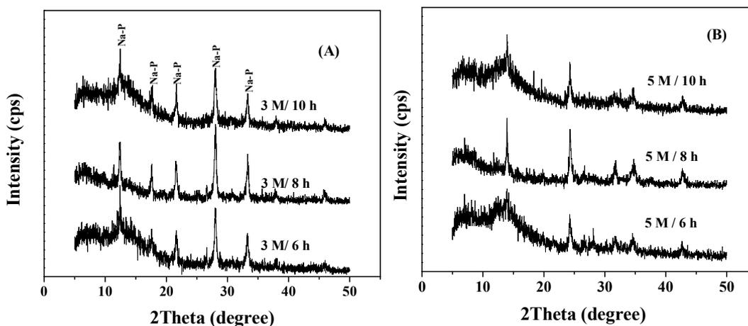
Fig. 4 X-ray diffraction patterns of the products obtained at various times
