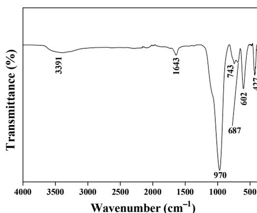
Fig. 6 FTIR spectra of the synthesized Na-P zeolite
