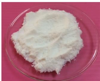
Fig. 1 Silica powder from sugarcane bagasse ash
