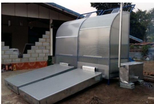
Fig. 2 The pictorial view of a small-scale greenhouse solar dryer
