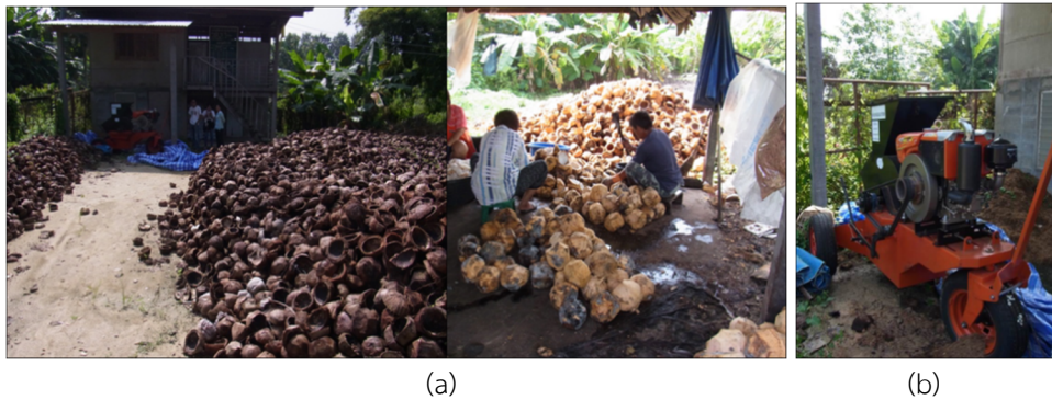
Fig. 1 (a) Coconut shells and (b) Multi-shredding machine employing a diesel engine
