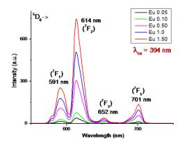
Fig.6 The emission spectra for LGBO glasses doped with different mol% of Eu<sup>3+</sup>
