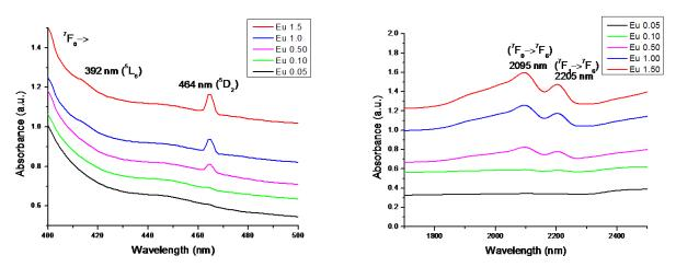
Fig. 2 The absorbance spectra for LGBO: Eu<sup>3+</sup>glasses in VIS range
