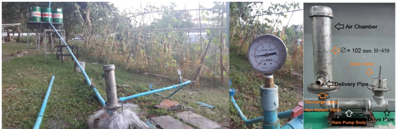
Fig. 2 The operation of hydraulic ram pump
