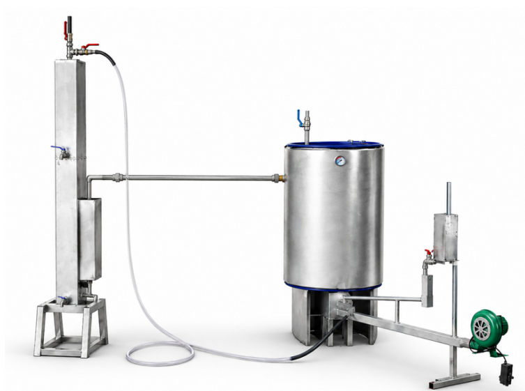
Fig. 2 Photograph of the fabricated prototype of the community-scale single-pillar pyrolysis reactor.
