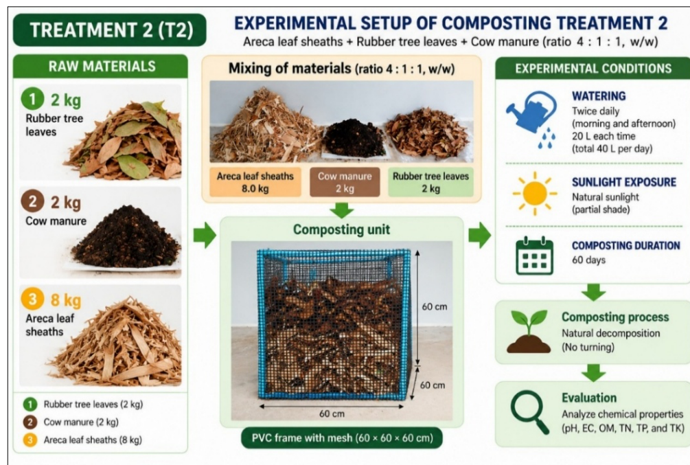
Fig. 3 Procedure for adding materials to the treatment 2 (T2) composting cage.
