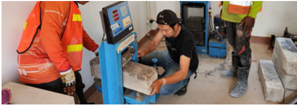
Fig. 5 Flexural strength test
