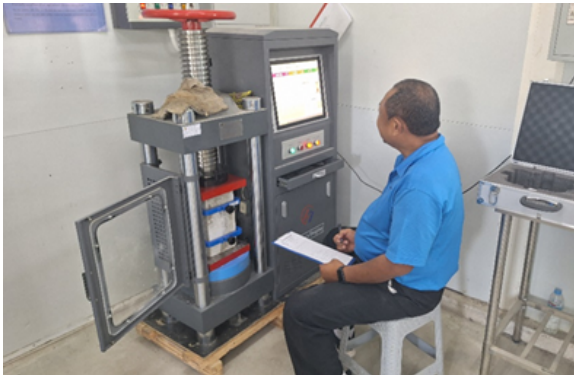
Fig. 6 Measured modulus of elasticity of concrete
