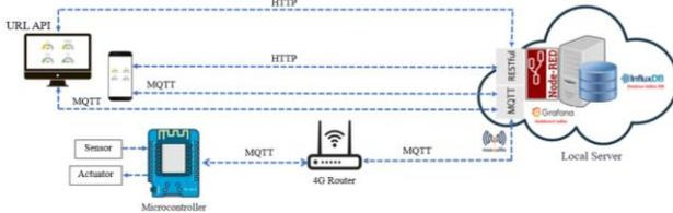
**Fig. 2** The block diagram of the proposed system.
