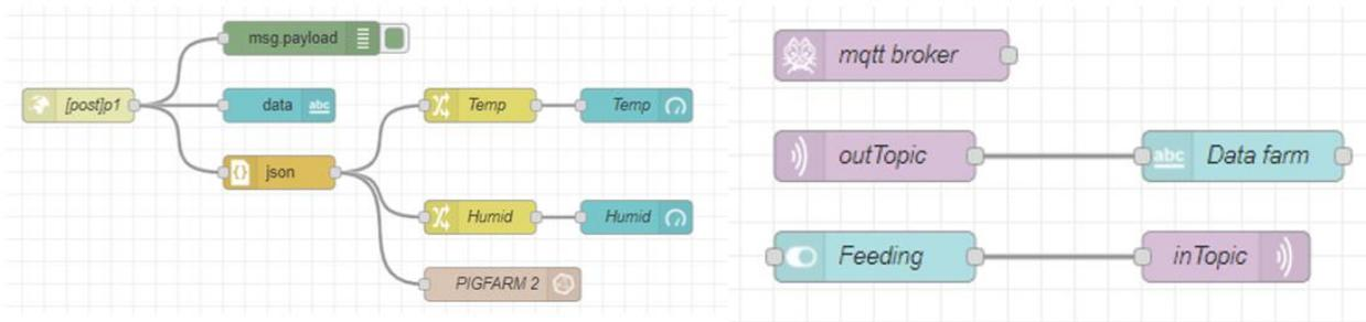
**Fig. 5** The Node-RED management page (a) NoSQL databased flow and (b) MQTT protocol.
