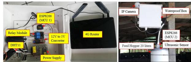
**Fig. 6** Installation the IoT nodes in the pig farm.
