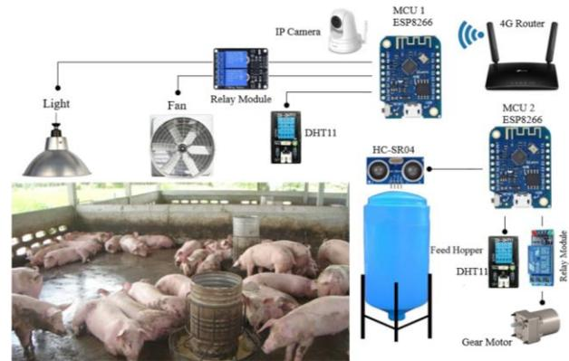
**Fig. 3** The diagram of the IoT nodes.
