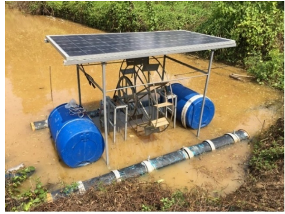
Fig. 1 A small water turbine integrated with a solar panel 330 Wp type of poly crystalline.
