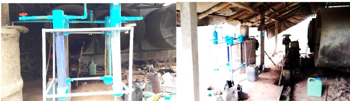
Fig. 2 A small biogas purifier used for upgrading the engine fuel in the evaporative conditioning system
