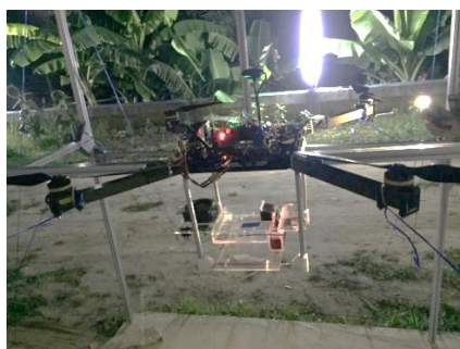
Fig. 1 a drone together with the fertilizer-in-bubble releasing system installed
