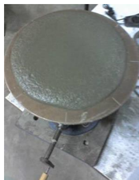
Fig.2 Flow table test according to ASTM C230
