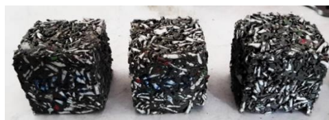
Fig.3 Samples of mortar for compressive strength tested using ASTM C109/C109M
