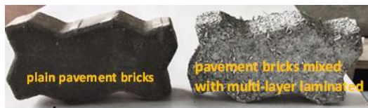
Fig.4 Samples of plain pavement bricks and pavement bricks mixed with multi-layer laminated scrap.
