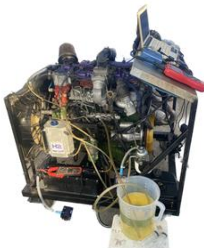
Fig.3 Isolating hydrogen from water for use in a diesel engine of 2500 cc.
