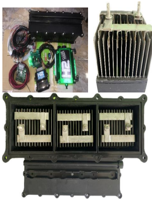
Fig.2 Small hydrogen gas separator from water complied with 2,500 cc engine.
