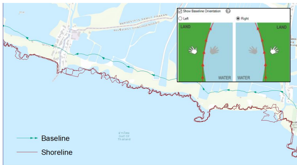
Figure 8. Baseline orientation using in attribute table.
