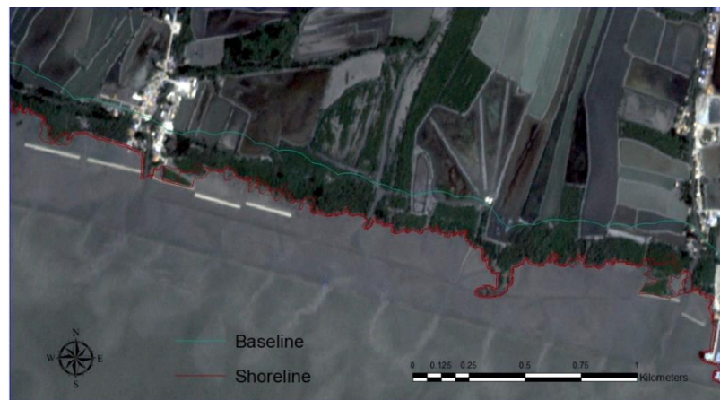
Figure 7. Baseline and shorelines using in DSAS calculation process.
