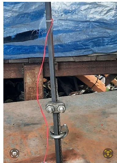
Figure 12 Installation characteristics of the strain gauge, steel rod, and wire rope.
