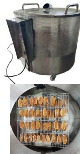
Figure 2 Experimental setup test with a banana fruit.
