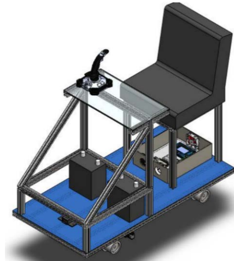
Figure 1 Model of the structure and equipment of the geometry inspection vehicle.
