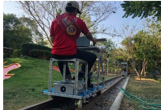
Figure 13 The testing of measurements for the width, incline, and cross-level height of the railway.
