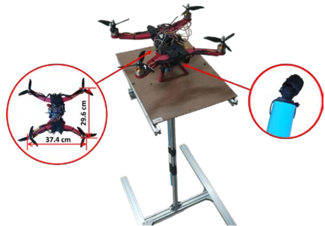
Figure 8 The drone is mounted onto the test stand.
