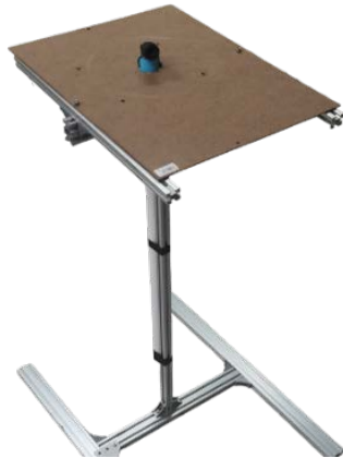
Figure 6 Drone mounting base for flight testing.
