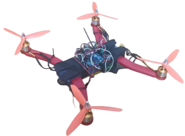
Figure 2 UAV (Drone) from PLA material.
