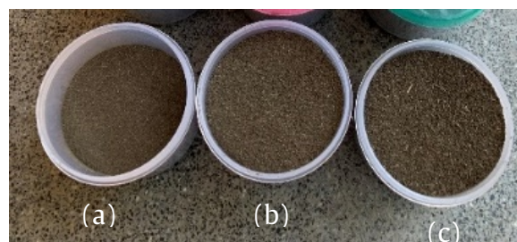
Figure 2 Filter cake residue with different particle sizes of (a) 20, (b) 60, and (c) 100 mesh.
