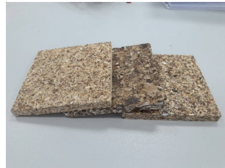
Figure 1 Characteristics of wood substitute materials from rhizomes and cassava peel.
