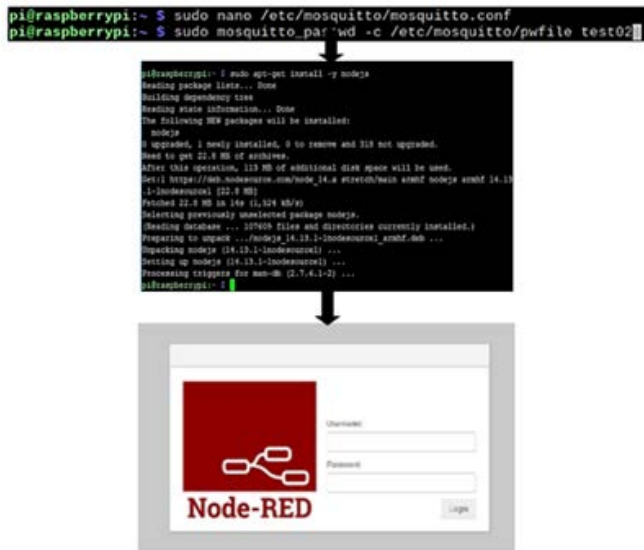
Figure 2 Node-RED uses the cloud server on Raspberry Pi.
