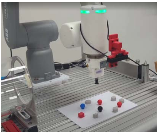
Figure 1 Cobot is equipped with an eye-on-hand camera to be used in this study of pick-place operations.
