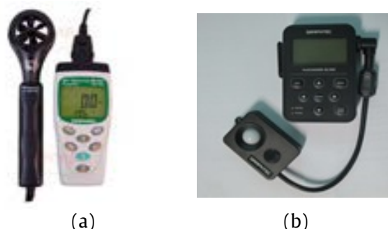
Figure 2 (a) Air velocity meter; (b) Illumination and solar sensor.
