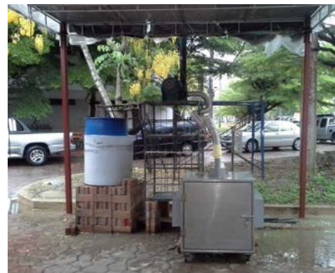
Figure 7 Using a blower to draw hot air to use in baking.
