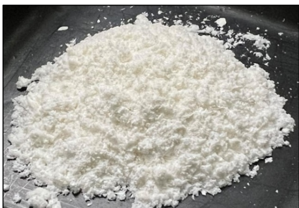
Figure 6 The Characteristics of 2-KGA powder after activated carbon adsorption and crystallization by freeze-drying.
