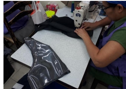
Figure 2 Sewing the body of ballistic vest.
