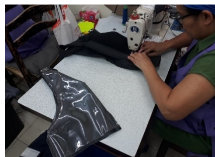
Figure 2 Sewing the body of ballistic vest.
