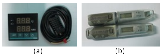
Figure 1 (a) Measurement and temperature control; (b) Temperature and Humidity sensors and data-logger.
