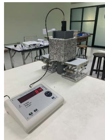
Figure 2 Experimental setup for gamma-ray shielding measurements using a Co-60 source and a Geiger-Muller detector. The system was used to measure incident and transmitted count rates for evaluating the shielding performance of the concrete samples.
