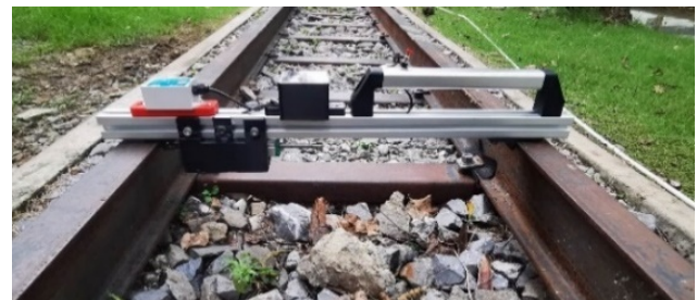
Figure 14 The measuring instruments used to compare the measurements of gauge width and angle of inclination.
