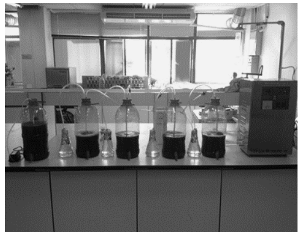
Figure 2 Wastewater treatment using the ozonation process.
