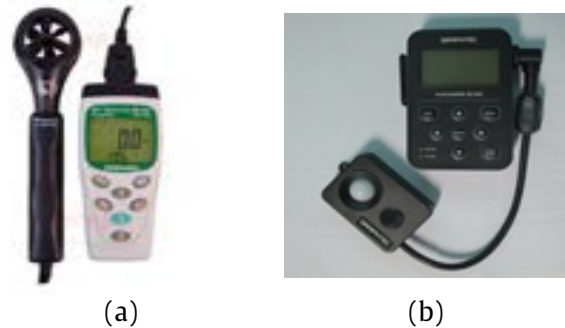
Figure 2 (a) Air velocity meter; (b) Illumination and solar sensor.
