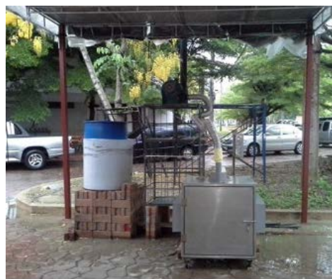
Figure 7 Using a blower to draw hot air to use in baking.
