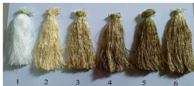
Figure 8 Color appearance of dyed Eri silk fabrics in various solvents; (1) non-dyed Eri silk fabrics (2) water, (3) EtOH/water (25: 75), (4) EtOH /water (50: 50), (5) EtOH /water (75: 25), and (6) EtOH.
