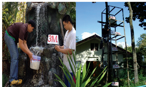
Figure 2 Data collection of water inlet flowrate at various supply head, discharge volume and 10 m delivery head
