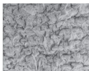
(d) fabric made from MC with 3.5 cm fiber spun yarn
