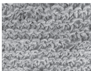
(a) fabric made from MH with 2 mm strip spun yarn
