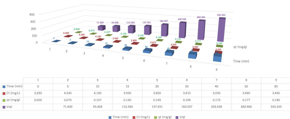
Figure 6 Pseudo-second-order kinetic model of coconut-shell activated carbon for wastewater treatment.
