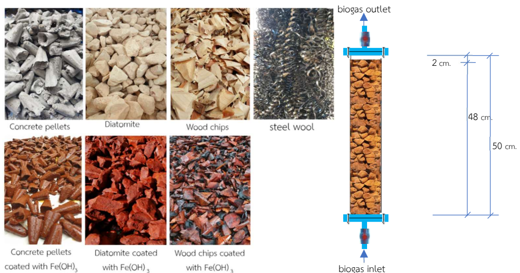
Figure 1 Adsorbent material (left) and design of fixed-bed adsorption column (right) used in the experiments.
