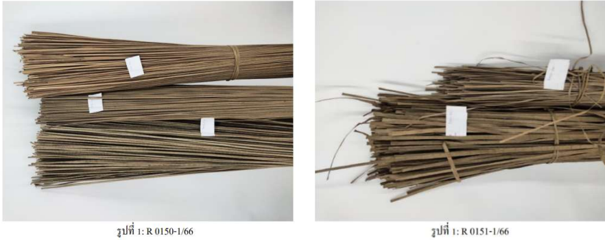
Figure 4 Dried krajoed strands coated with mud (Left) and extruded krajoed strands (Right)
