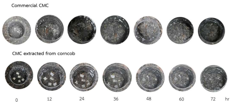
Figure 2 Appearance of CMC film before and after with soil embedding methods
