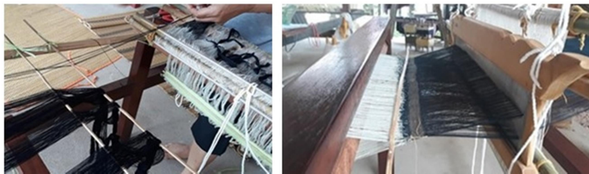
Figure 8 Process to each thread of the warp passes through in a heddle
