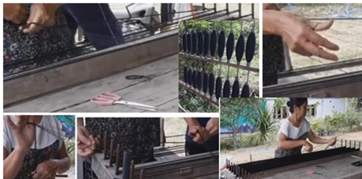
Figure 6 Process to threads pattern arrangement by heddles
