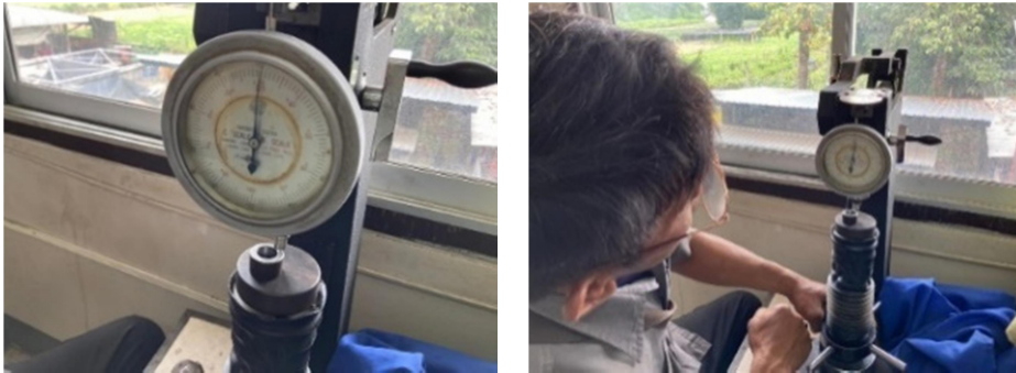
Figure 8 The hardness test in Rockwell (HRC)
