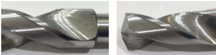
Figure 4 Drill bit after forming
