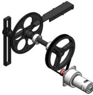
Figure 2 Power transmission for biomass feeder
