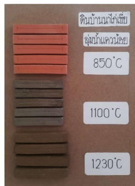
Figure 4 Baked mud rod at various temperatures . (850°C , 1,100°C and 1,230°C)
