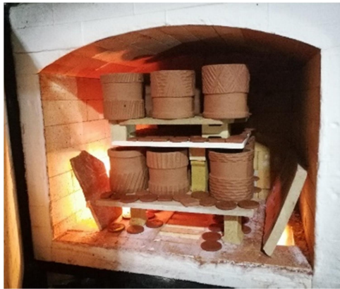
Figure 9 Firing at temperature at 1100 degree Celsius.
