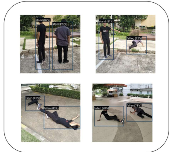
Figure 10 Simultaneous detection of falls across multiple individuals with varying statuses.
