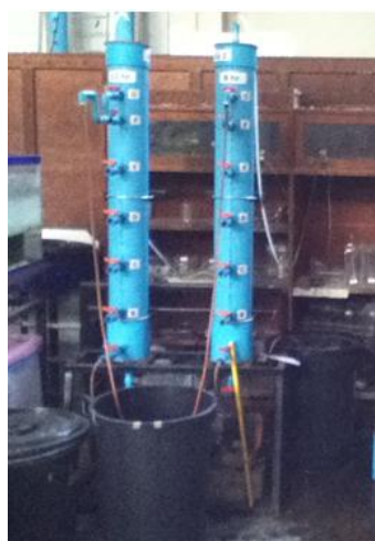
Figure 2 Utilized upflow anaerobic filter system in the Experiments
