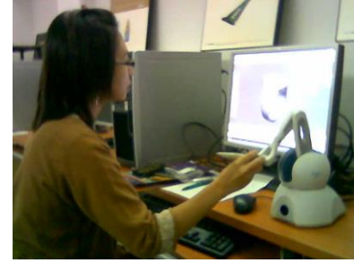
Figure 2 The use of haptic device in product modeling
