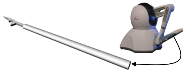
Figure 7 The simulated carving tool handled by using the stylus of PHANTOM haptic device
