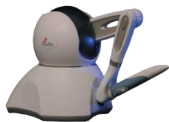
Figure 1 An example of commercial haptic device (PHANToM Omni) developed by SensAble Technologies [5]
