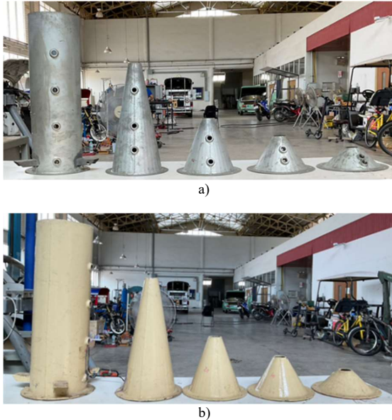
Figure 6 Laboratory-scale silos: a) Steel silo b) Fiberglass silo.
