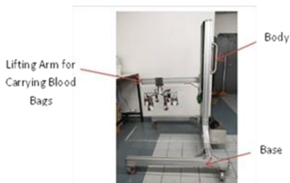
Figure 8 Parts of the Vertical Lifting Device
