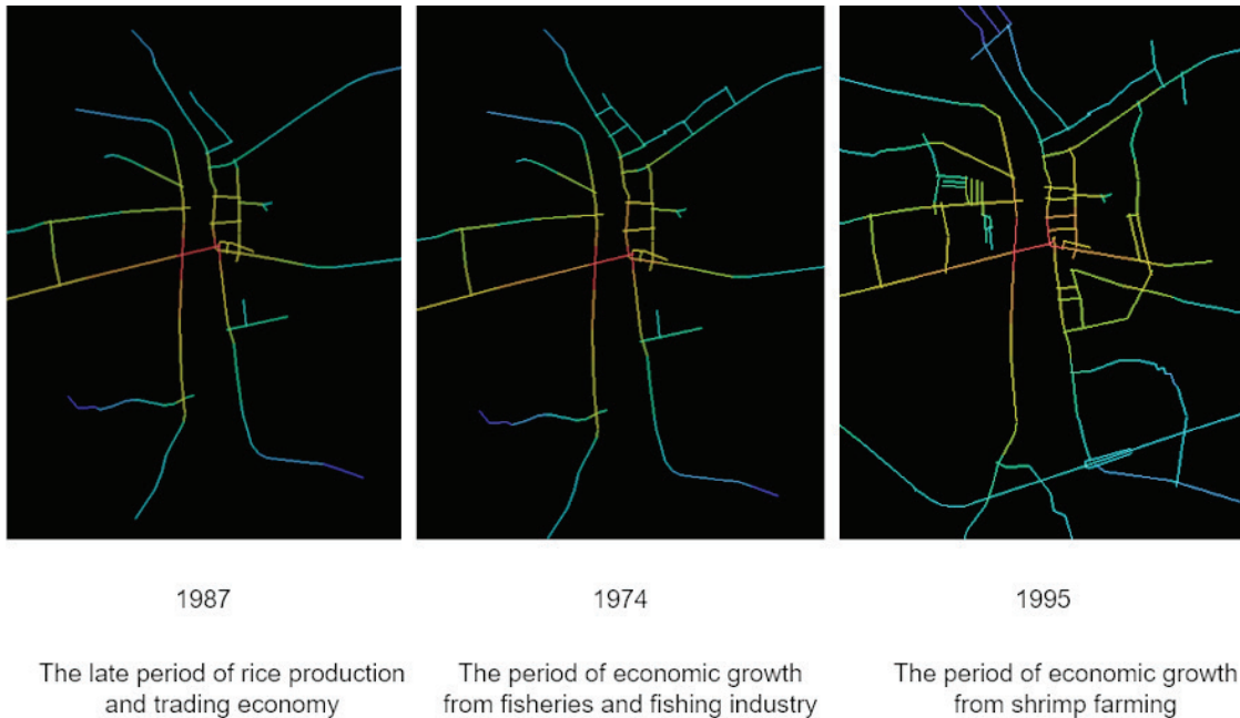
Figure 3: The analysis of the accessibility of transport network and city public space (Global Integration (RN)) using Space Syntax technique, in 1967, 1974 and 1995.
