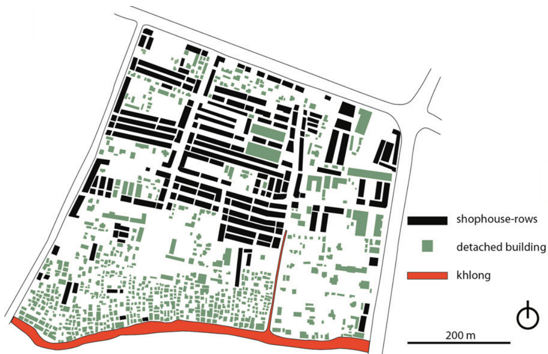
Figure 5: The land based shophouse-rows and the detached houses and high-rise are the usual building blocks of the terrestrial urban structure in Bangkok
