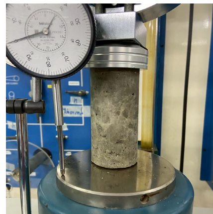
Figure 3 Testing specimen before the compressive strength test.
