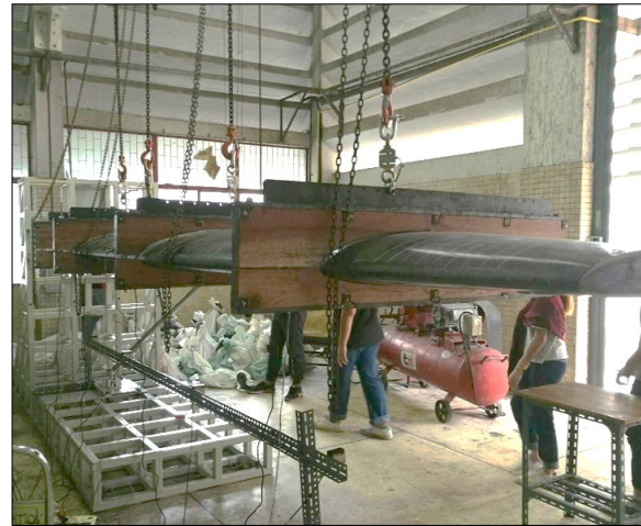
Figure 1 Shows wing structural testing process
