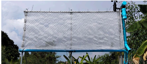
Figure 5 Physical implementation of the integrated fog trap and atmospheric water production system in a highland field environment
