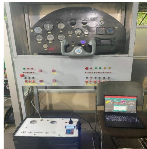
Figure 9 Air Data Test Set Implementation with Instrument Panel
